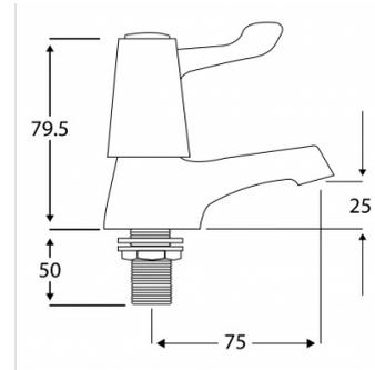
Lever operated basin taps for connecting to hot and cold water. Manufactured from chromium plated brass. Conforms to BS5412 standard.
